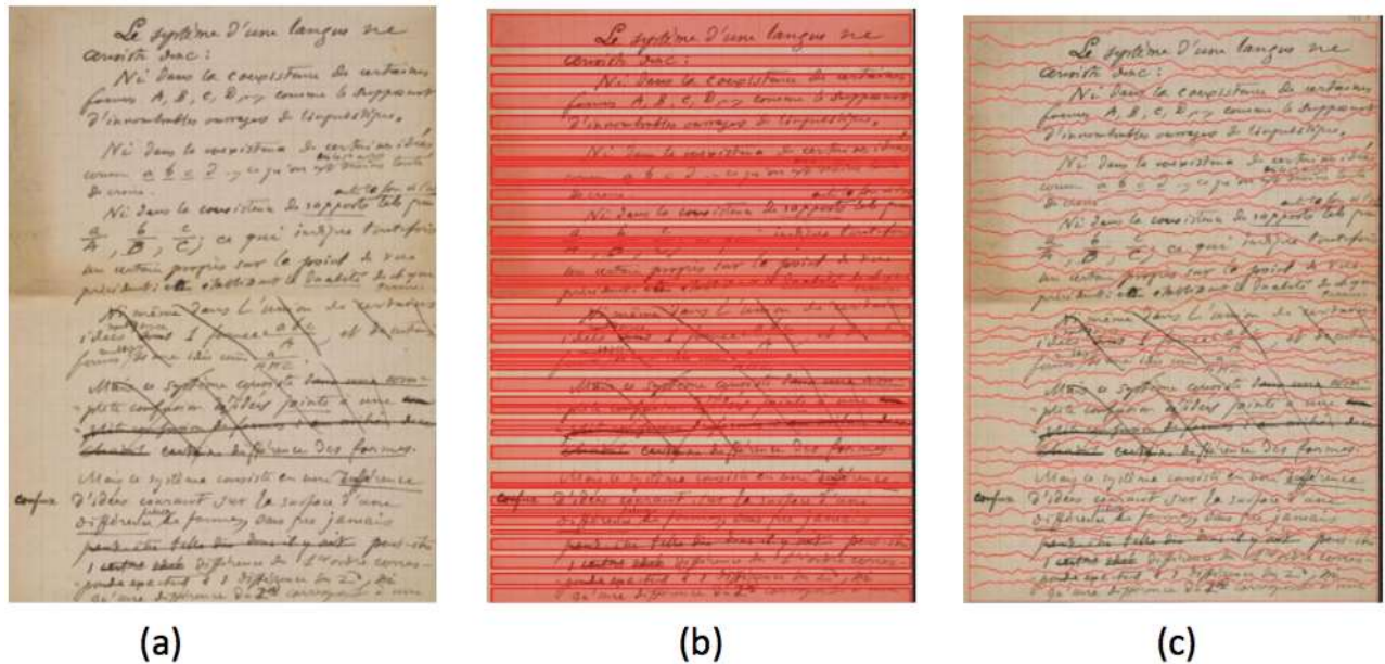
Figure 3 The results of two different text line extraction methods. The original images have been cropped for size reasons. (Bibliothèque de Genève, BGE_AdS_372_5_f171)
